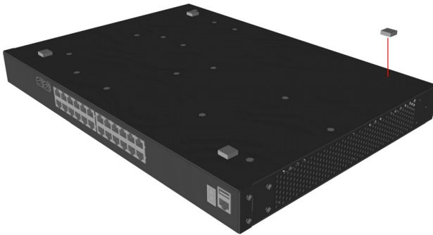
Figure 15: Attaching the Adhesive Feet
